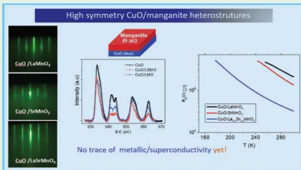
Fig.: Left: RHEED diffraction image for CuO (4 uc)/ manganite (6 uc) indicating a 2D growth pattern. Middle: the Cu 2p core-level XPS spectrum indicating Cu<sup>2+</sup> state in CuO, though the satellite peak intensity seems to diminish with manganite interfacing (a careful analysis is being carried out). Right: Sheet Resistance vs temperature for various CuO / manganite heterostructure exhibiting insulating trend. (Fig. of Sec.-h)
