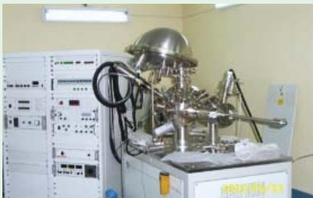
The present XPS system has a dual X-ray Aode (Mg/Al). The sample can be aligned by a manipulator. Photoelectrons are energy analyzed by a hemispherical mirror analyzer. The system also has the facility for sample annealing and Ar ion sputtering. Sputtering technique can be utilized for doing depth profiling studies. All the experiments are carried out under ultra high vacuum (UHV) conditions at the vacuum of  $1 \times 10^{-10}$  Torr.
