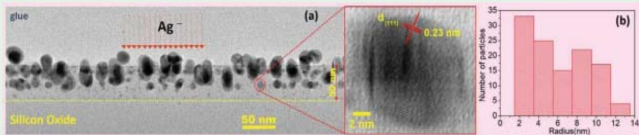
(a) The-cross sectional TEM image of the silver implanted  $\text{SiO}_2$  film/ $\text{Si}(100)$ . The red arrows show the direction of silver ion implantation. Towards the right, the high resolution image shows the single crystalline nature of the formed Ag nanoparticles. (b) The corresponding size distribution of the Ag nanoparticles. (Fig. of Sec-E)
